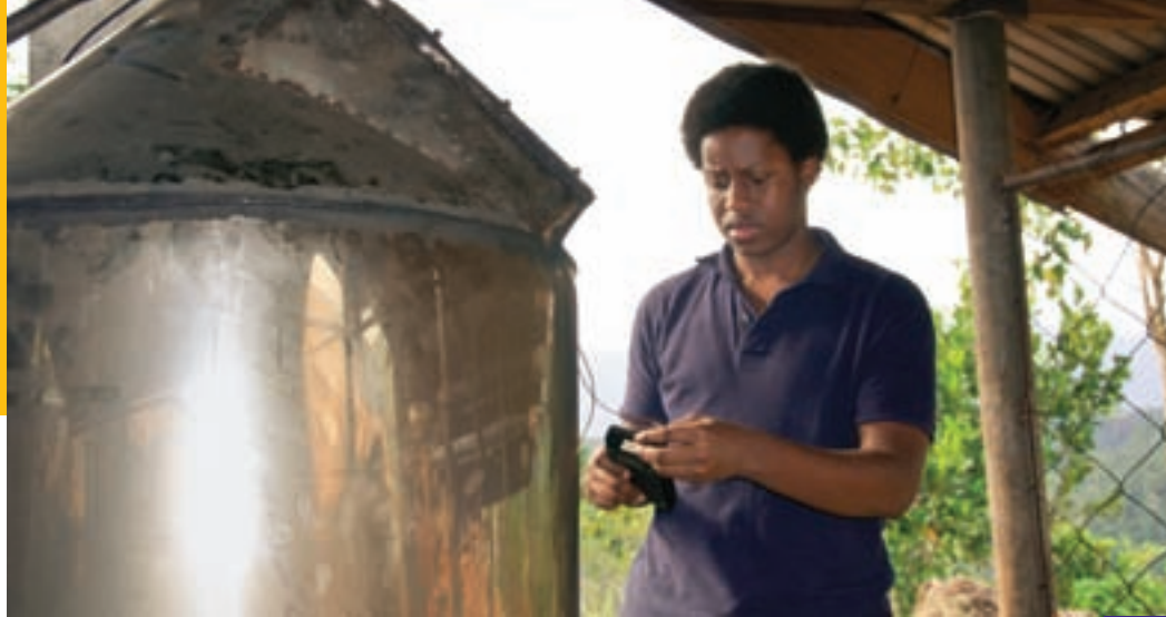
Dalmas Wambura ME '10 and current graduate student in the Chemical Engineering Department, reads temperatures from different probes located at varying levels in a lemongrass oil retort.
